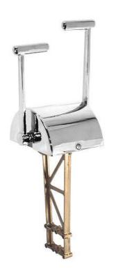
This control is available with three different handles; standard, handles with plastic grips or curved handles with knobs. An optional clutch and throttle interlock can be ordered with this unit. The purpose of this interlock is to prevent shifting, above engine idle. It is only available for systems having clutch and throttle on the same control. In two station applications only one interlock is required. For gears with an electric clutch, an adapter with two microswitches can be ordered.
