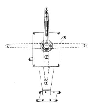
This control can be **ordered** (can not be changed in the field) with the neutral position of the handle in any one of the four positions indicated. Position "1" is standard. Please add appropriate number.
